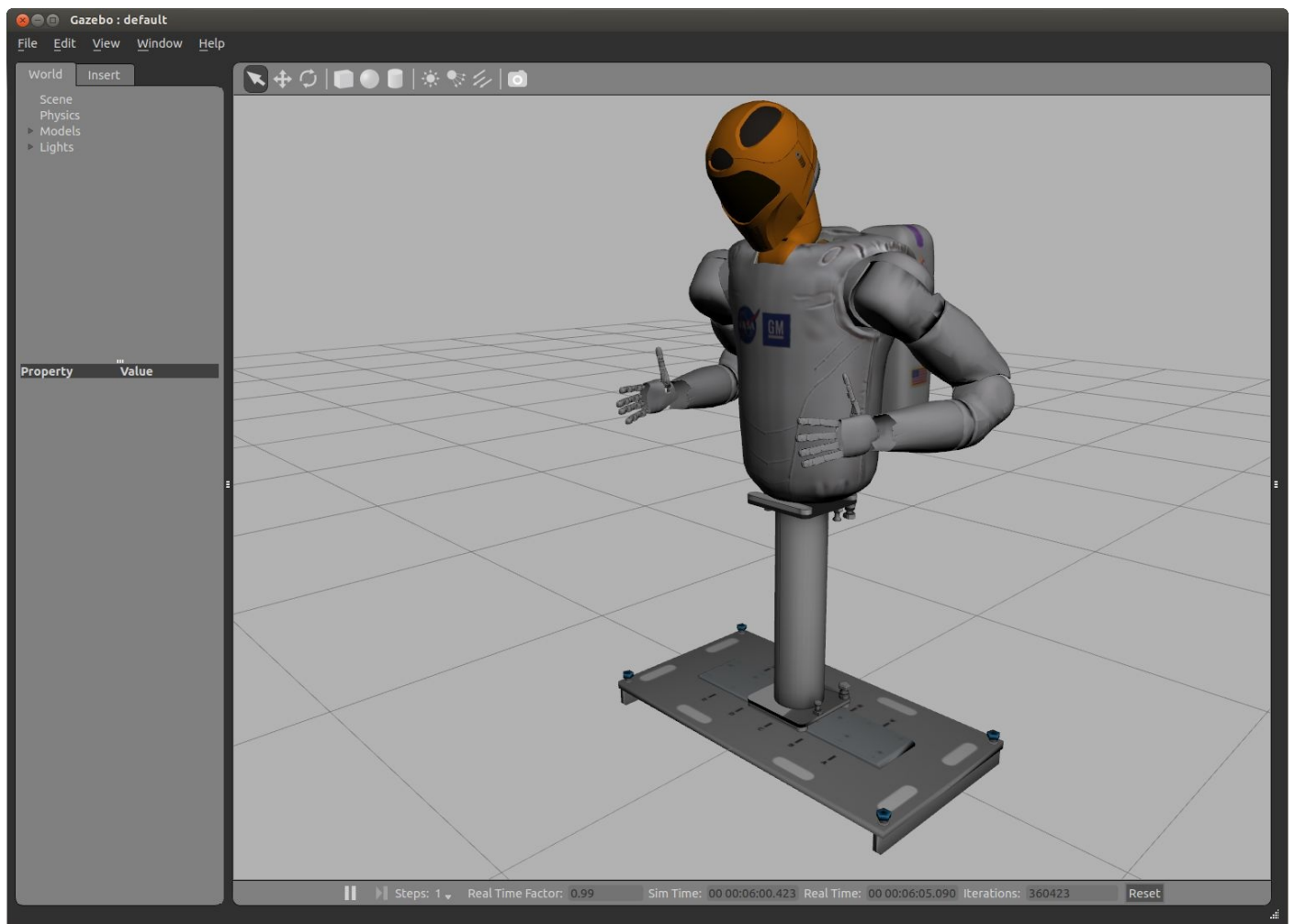
Figure 6-3. The NASA R2 robot running in the Gazebo simulator
