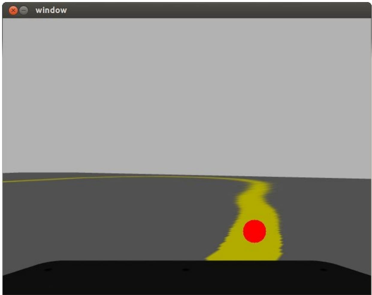
Figure 12-7. The original image with the red circle overlay, which shows the algorithm's estimate of the center of the line
