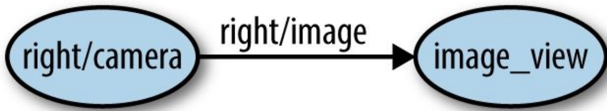
Figure 2-9. Image topic has right/image using command-line remapping
