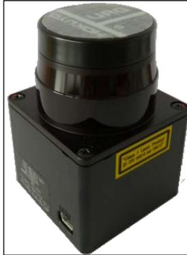
The Hokuyo URG-04lx model is a low-cost rangefinder commonly used in robotics. It has a very good resolution and is very easy to use. To start with, we are going to install the drivers for the laser:
