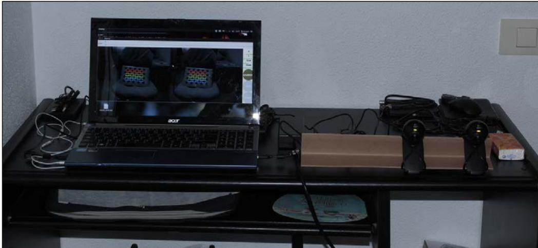
The calibration is done by the same `cameracalibrator.py` node used for monocular cameras. We pass the left-hand side and right-hand side cameras and images, so the tool knows that we are going to do stereo calibration. The following is the node in the launch file:
