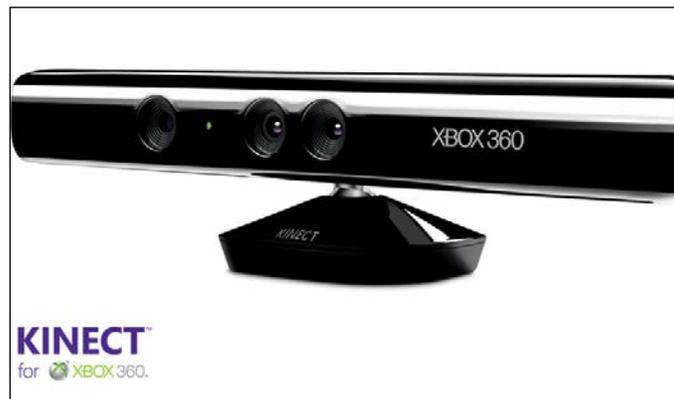
In ROS, we are going to use two of these sensors: the RGB camera and the depth sensor. In the latest version of ROS, you can even use three.
